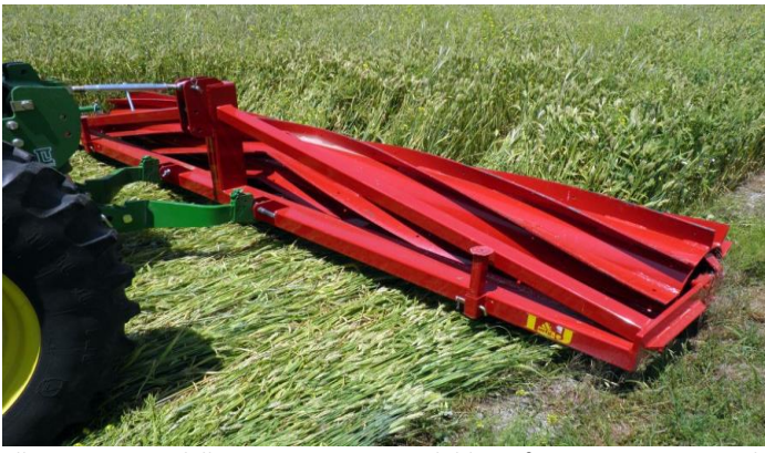
Roller crimpers to kill cover crops are available as front or rear mounted models.
